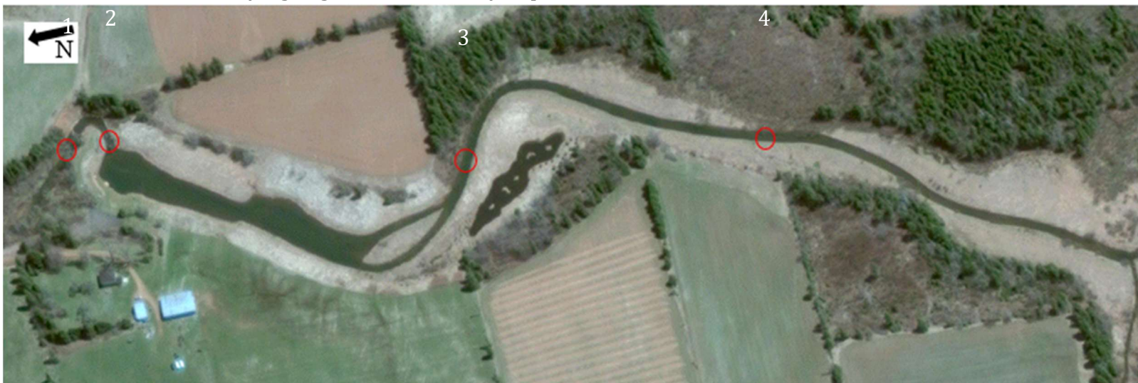
Figure 4: Macroinvertebrate Sampling Areas Along Rackham's Pond on the Wheatley River, Each Location one Hester-Dendy Sampler was Placed.
